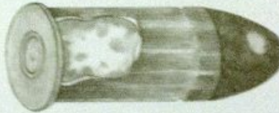
Primer ignites powder charge, forming gases
