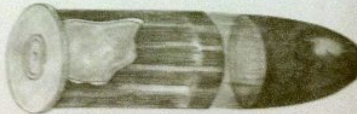
Primer ignites powder charge, forming gases
